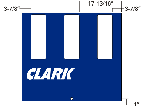
1CKWV3 42" (W) x 37-1/4" (H) x 1" (D) Wayne Vista 3-Hose (Full Height. No Totalizer Slots) Qty. _____ Pair
